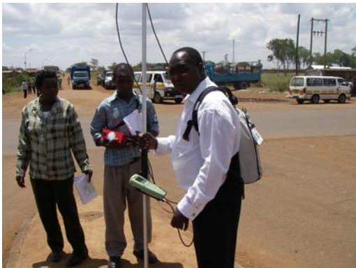
Data collection using RTK GPS receiver
